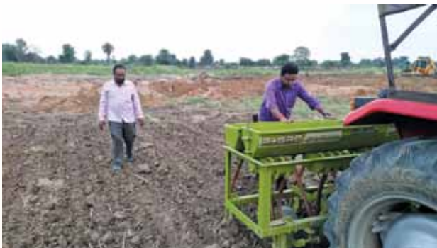
(a) Sowing with zero-till ferti-seed drill machine
