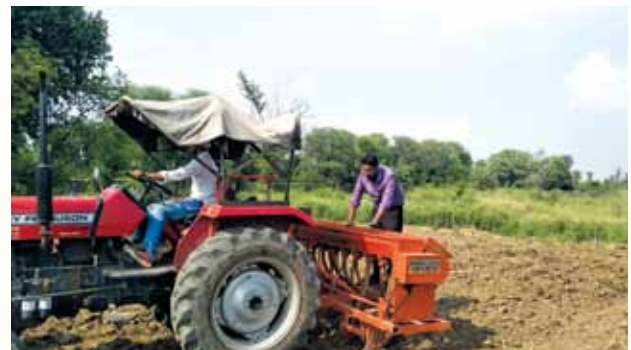
(b) Sowing with multi-crop seed-cum fertilizer drill machine
