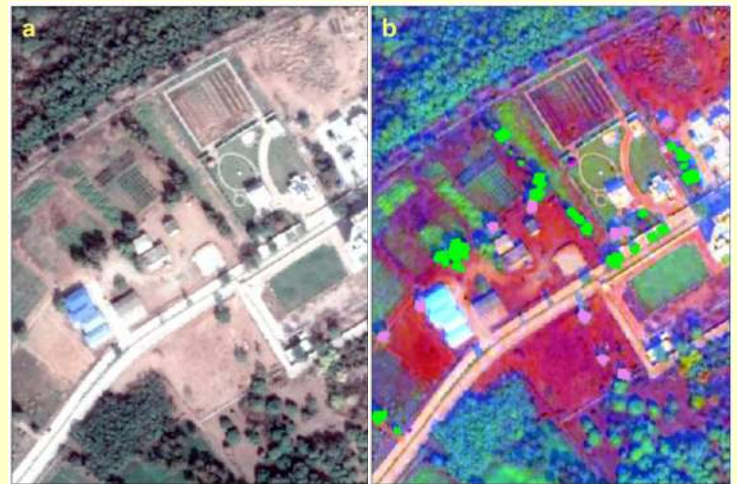
Fig. 1: Instance segmentation using the tree dataset. (a) Initial image in its natural colour (b) PCA image with individually labelled tree crowns.
