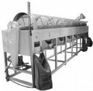
Raw cashew nut grading machine
